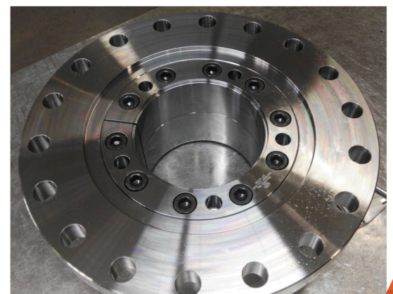
Fig. 10 Re-assembling of each coupling half after step 11
